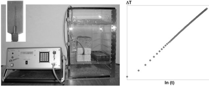
Figure 3. Measurement of thermal conductivity at dry state – left : CT Meter, Hot wire and dry chamber, right : experimental thermogram
