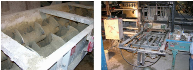
Figure 2. Precasting method (left : mixer, right : block press)
